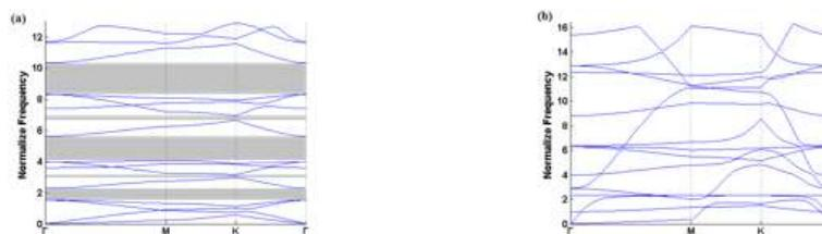
Fig. 1 Dispersion relations of honeycomb structures with (a) curve beam ligament. (b) straight beam ligament.
