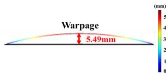
Fig. 2: Strip warpage of simulation result.
